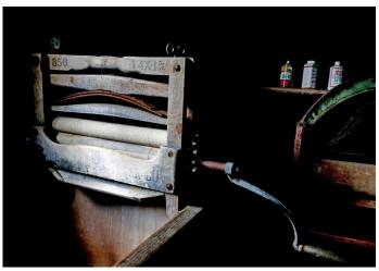
actually still work and the rollers are in good condition – damaged rollers will be less efficient, and can even damage your clothes.
